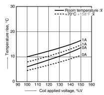
7. Ambient temperature characteristics Tested sample: TXS2-4.5V, 5 pcs.
