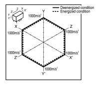
9-(2). Malfunctional shock (latching) Tested sample: TXS2-LT-4.5V, 6 pcs.
