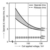
5-2. Operate & release time (with diode)
