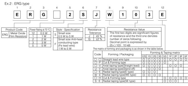
The above example 2 shows a small metal oxide film resistor, 2 W power rating, resistance value of 10 k $\Omega$ , tolerance ±5 %, and package of radial taping.
