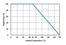
For resistors operated in ambient temperatures above 70°C, power rating must be derated in accordance with this curve.
