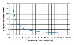
This graph indicates the amount that the rated power (at  $20^{\circ}$ C) of the standard HS Series resistor may be increased for overloads of 100mS to 60S
