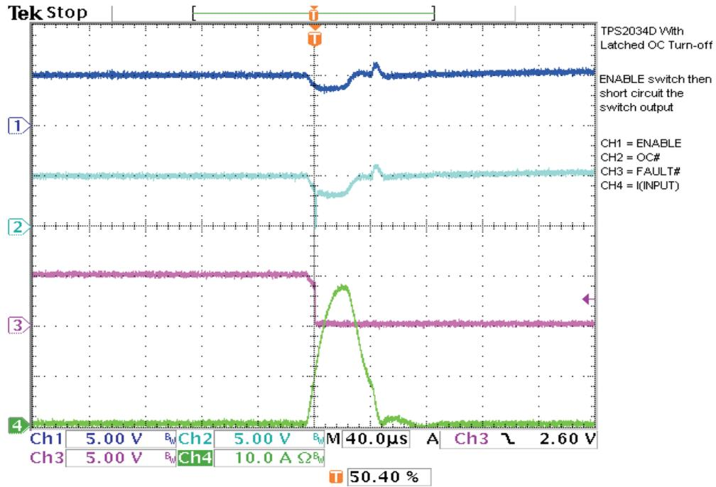
Figure 4. Enabled-Switch Output Is Short Circuited
