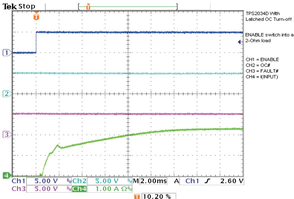
Figure 2. Switch Is Enabled Into 2- $\Omega$  Load
