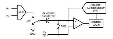
Figure 48. ADC102S021 in Hold Mode
