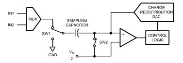
Figure 47. ADC102S021 in Track Mode
