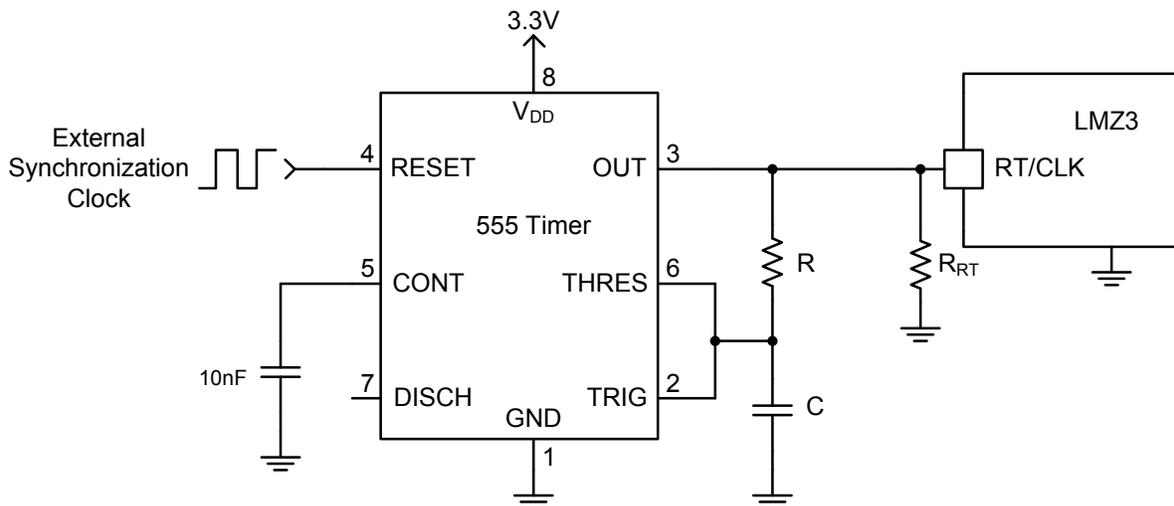
**Figure 1. 555 Timer Uninterruptible Clock Circuit**
