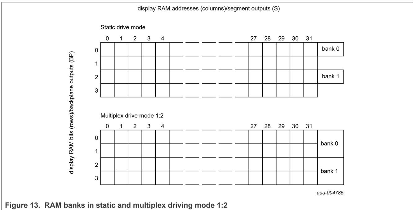
Figure 13. RAM banks in static and multiplex driving mode 1:2
