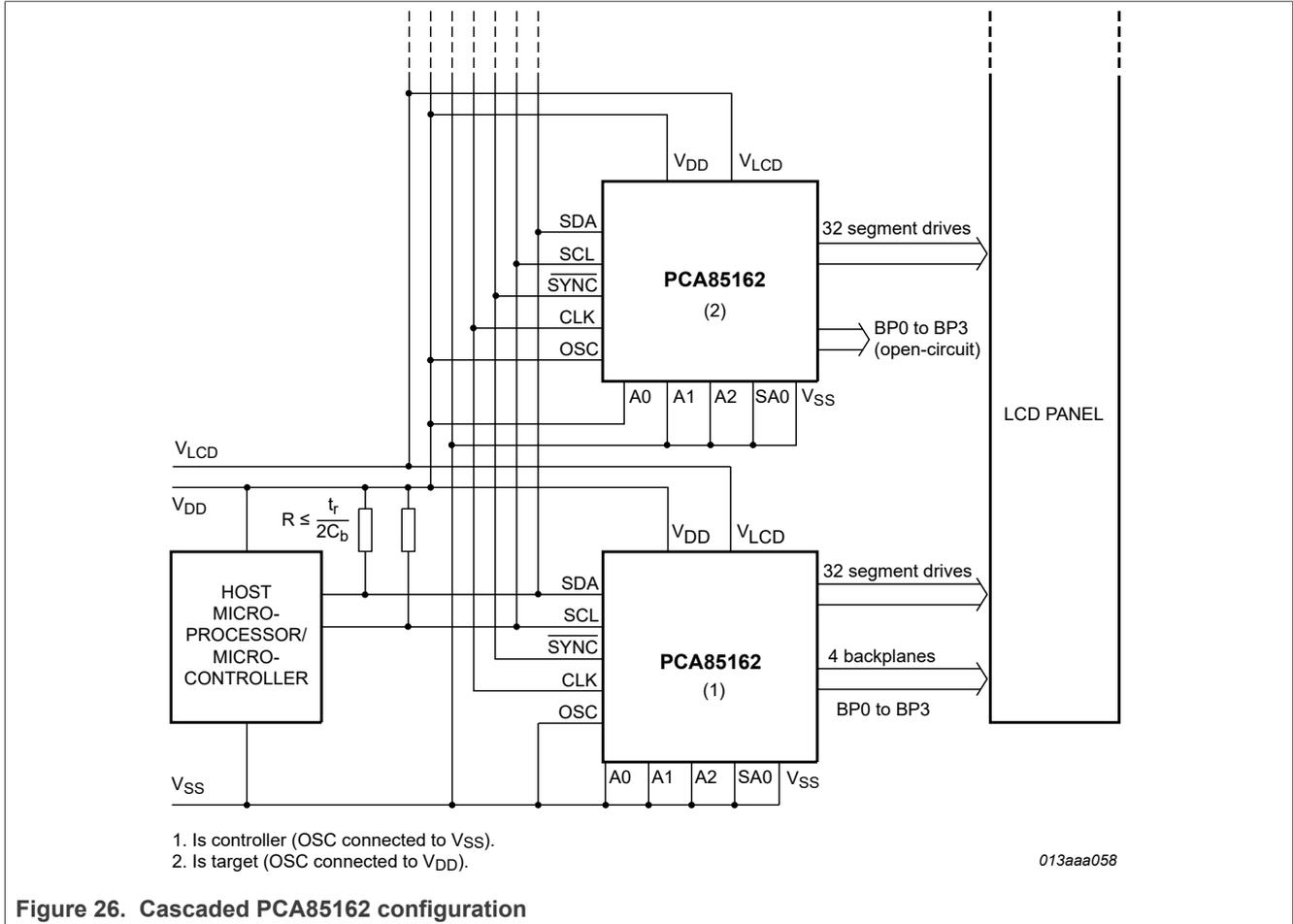
Figure 26. Cascaded PCA85162 configuration
