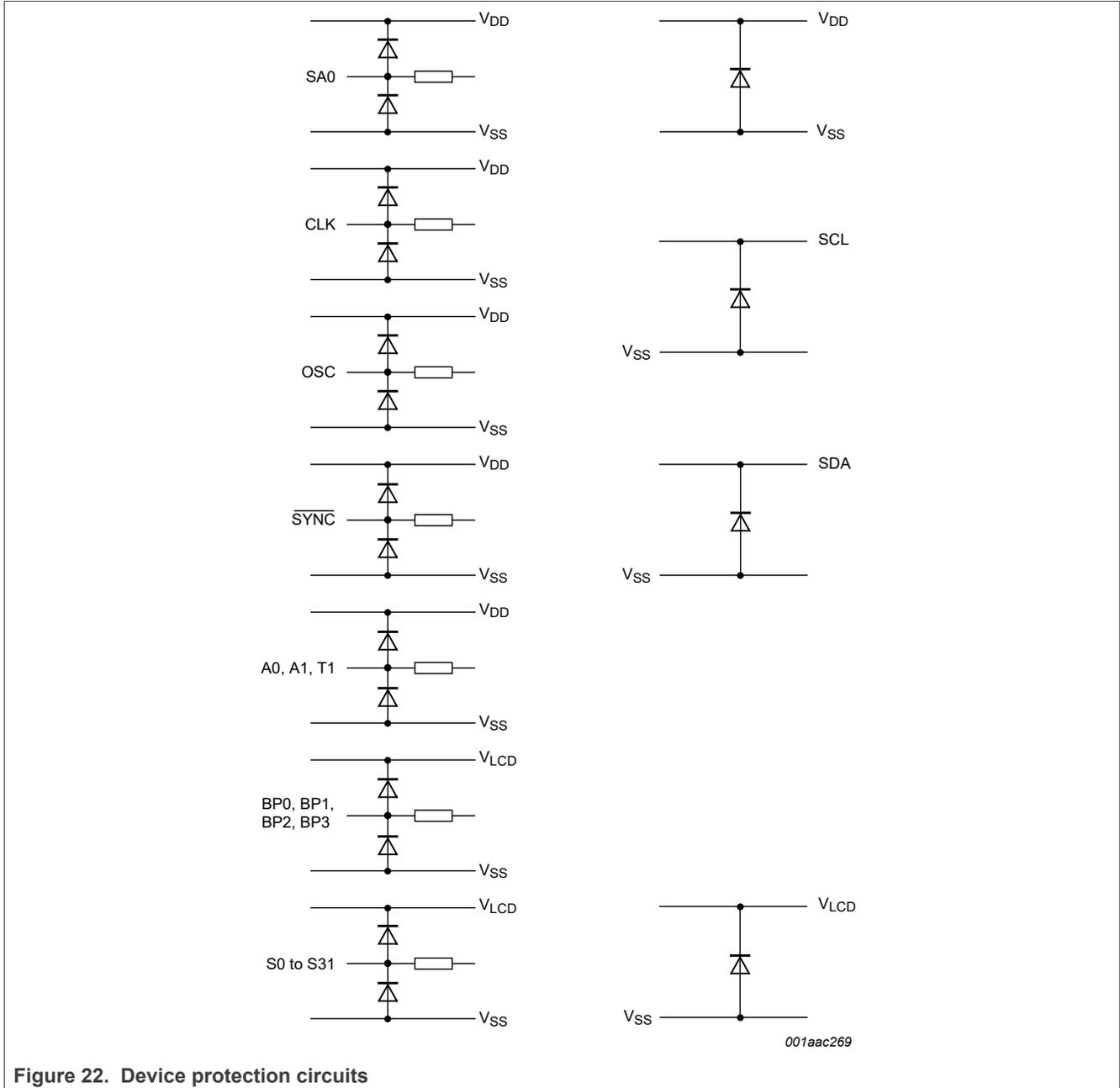
Figure 22. Device protection circuits
