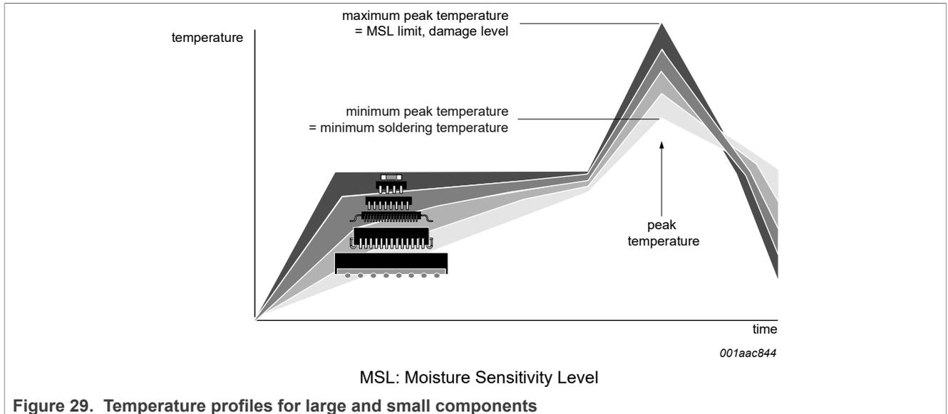
For further information on temperature profiles, refer to Application Note AN10365 “Surface mount reflow soldering description”.
