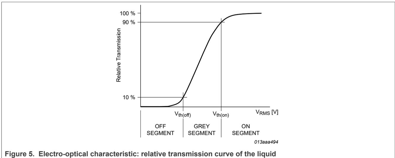
Figure 5. Electro-optical characteristic: relative transmission curve of the liquid
