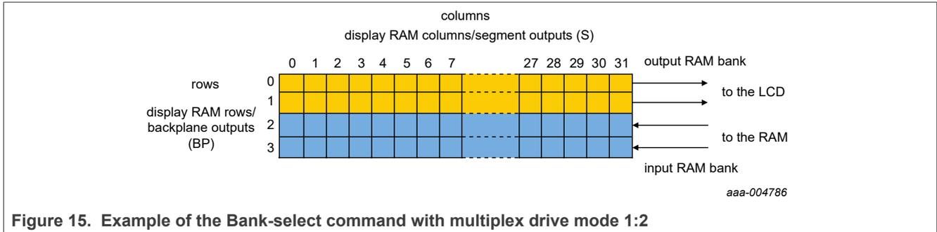
Figure 15. Example of the Bank-select command with multiplex drive mode 1:2
