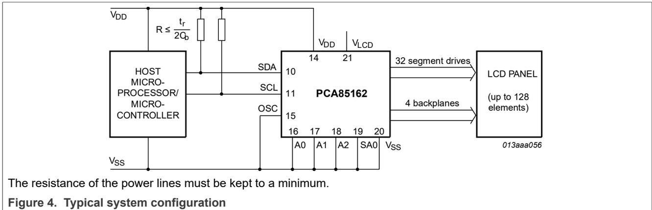
The host microcontroller maintains the 2-line I<sup>2</sup>C-bus communication channel with the PCA85162. The internal oscillator is enabled by connecting pin OSC to pin V<sub>SS</sub>. The appropriate biasing voltages for the multiplexed LCD waveforms are generated internally. The only other connections required to complete the system are the power supplies (V<sub>DD</sub>, V<sub>SS</sub>, and V<sub>LCD</sub>) and the LCD panel chosen for the application.
