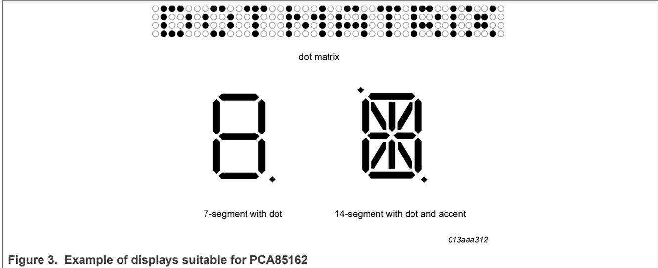
Figure 3. Example of displays suitable for PCA85162
