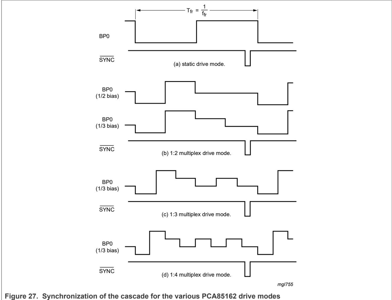
Figure 27. Synchronization of the cascade for the various PCA85162 drive modes
