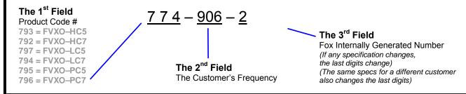
This example, FXO-PC726R-906 = LVPECL Output, Ceramic, 7 x 5mm Package, 2.5V, ±25 PPM Stability, -40 to +85°C Temperature Range, at 906 MHz
