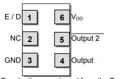
Terminations as viewed from the Top NOTE: XPRESSO LVPECL XOs are designed to fit on Industry Standard, 6 pad layouts
