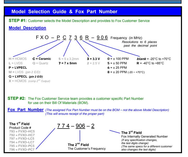
This example, FXO-PC736R-906 = LVPECL Output, Ceramic, 7 x 5mm Package, 3.3V, ±25 PPM Stability, -40 to +85°C Temperature Range, at 906 MHz
