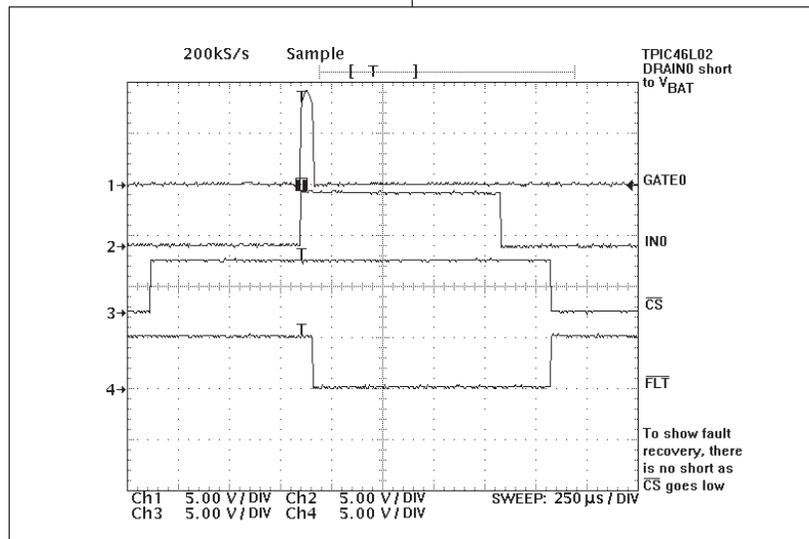
Figure 6. Fault Clears
