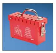
Group lock box is built with an exclusive tamper-resistant sliding lid design that keeps keys from being accessed until all padlocks are removed. Group lock boxes hold up to 13 padlocks.
