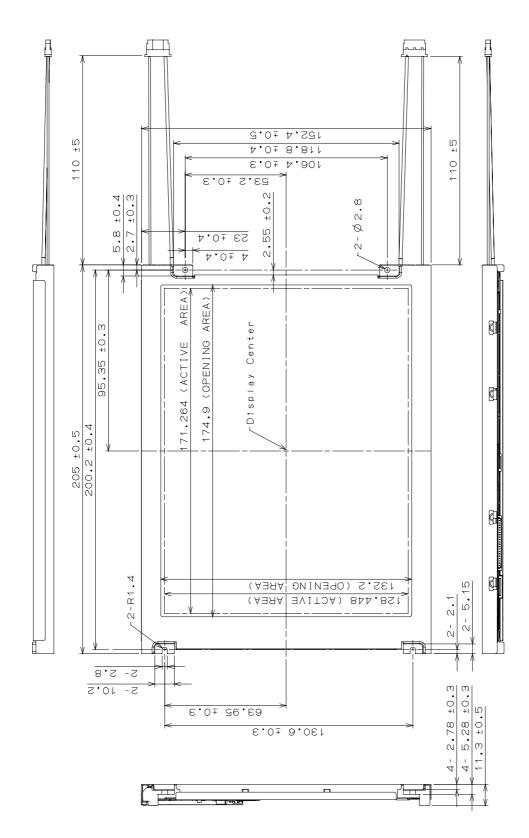
1)Tolerance is ±0.5mm unless noted 2)Except for thickness of PET film
