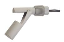
The RSF80 series are designed for mounting through the wall of a tank, via ½"NPT thread without requiring acces to the inside of the tank.
