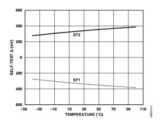
Figure 11. Typical Self-Test Change over Temperature
