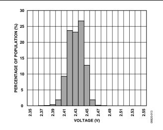
Figure 13. VTEMP Output at 25°C (VRATIO = 5 V)
