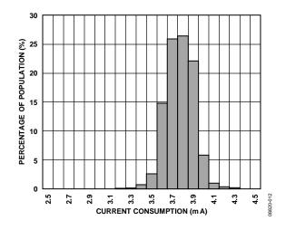
Figure 12. Current Consumption at  $25^{\circ}C$  (V<sub>RATIO</sub> = 5 V)
