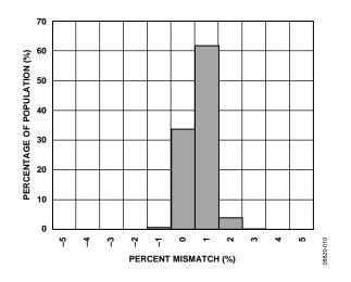
Figure 10. Self-Test Mismatch at  $25^{\circ}C$  (V<sub>RATIO</sub> = 5 V)
