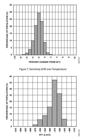
Figure 8. ST1 Output Change at  $25^{\circ}C$  (V<sub>RATIO</sub> = 5 V)
