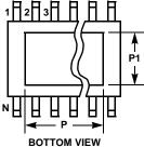
M24.173B 24 LEAD THIN SHRINK SMALL OUTLINE EXPOSED PAD PLASTIC PACKAGE
