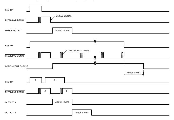
The hold pulse checks a system code of an initial single signal and a received signal and becomes "H" level only when data is valid.
