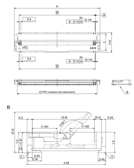
Notes  $\boxed{1}$  The coplanarity of each terminal lead is within 0.1 max.
