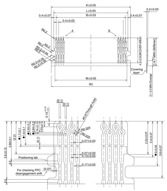
1 To prevent pattern cutting, when 4.7 mm or more of reinforecement film cannot be secured, make the overlap amount 0.5 mm or greater.
