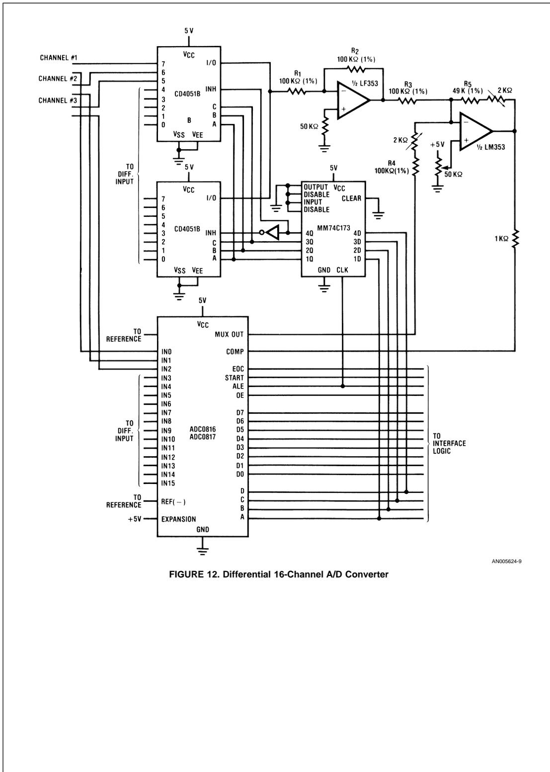
FIGURE 12. Differential 16-Channel A/D Converter
