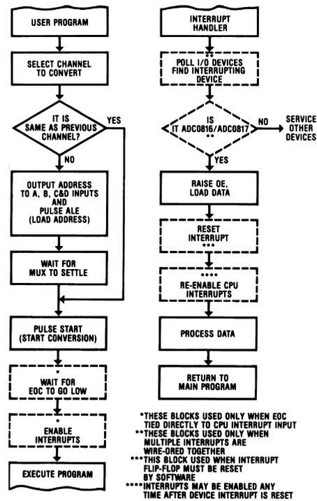
FIGURE 21. Flow Chart for Interrupt Control of ADC0816/ADC0817
