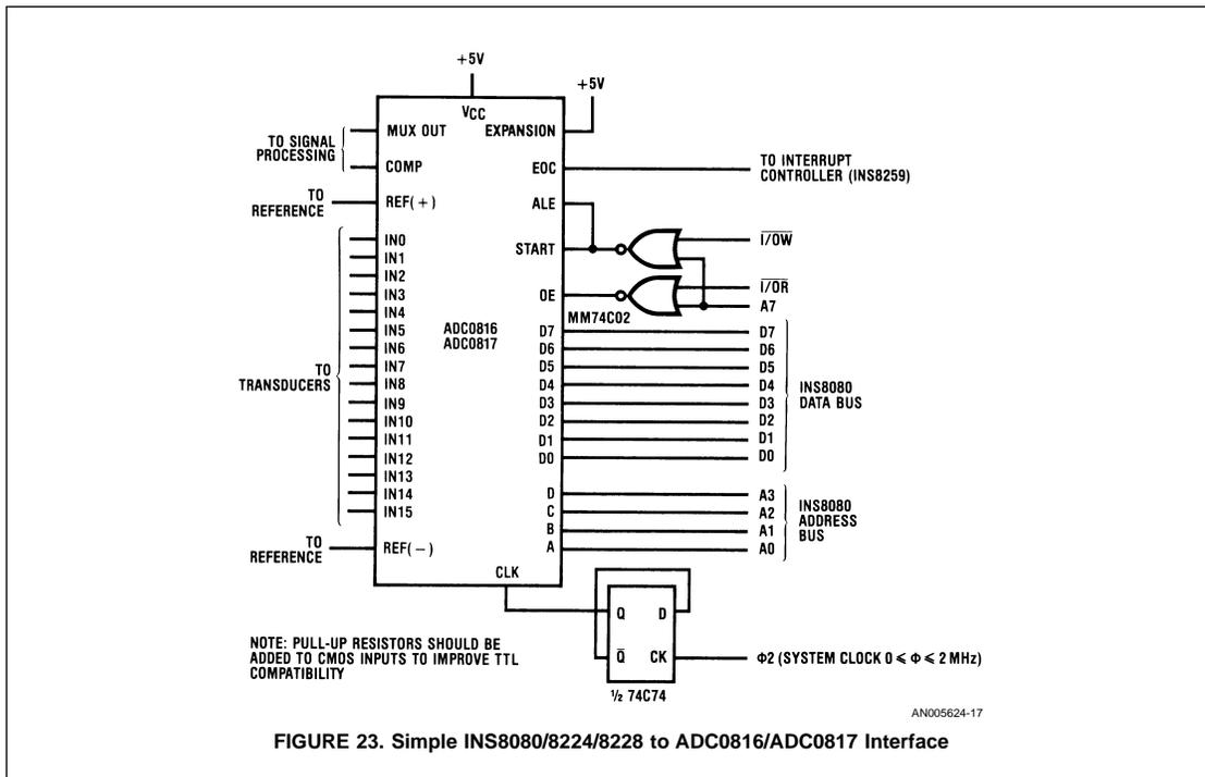
FIGURE 23. Simple INS8080/8224/8228 to ADC0816/ADC0817 Interface
