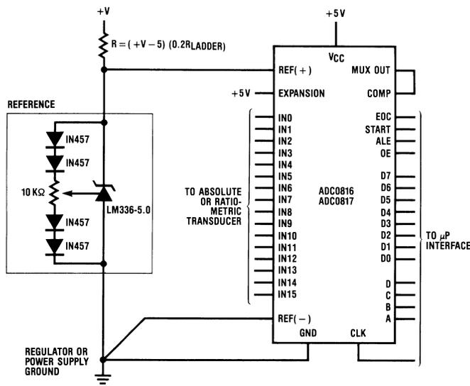
FIGURE 5. Simple Absolute Converter Using LM336-5.0 Converter
