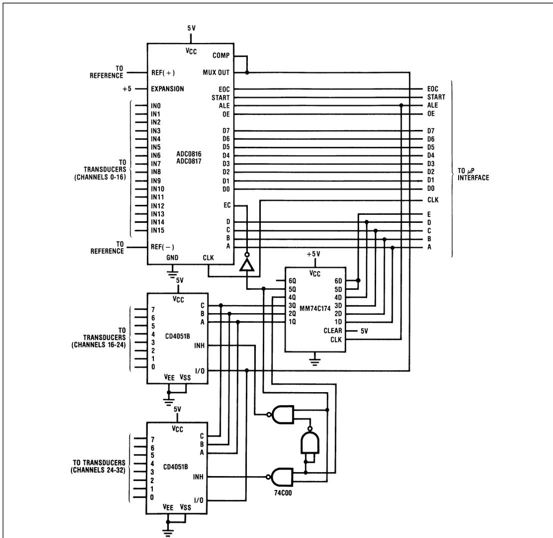
FIGURE 10. Simple 32-Channel A/D Converter
