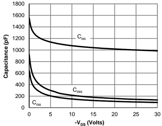
**Figure 8: Capacitance Characteristics**
