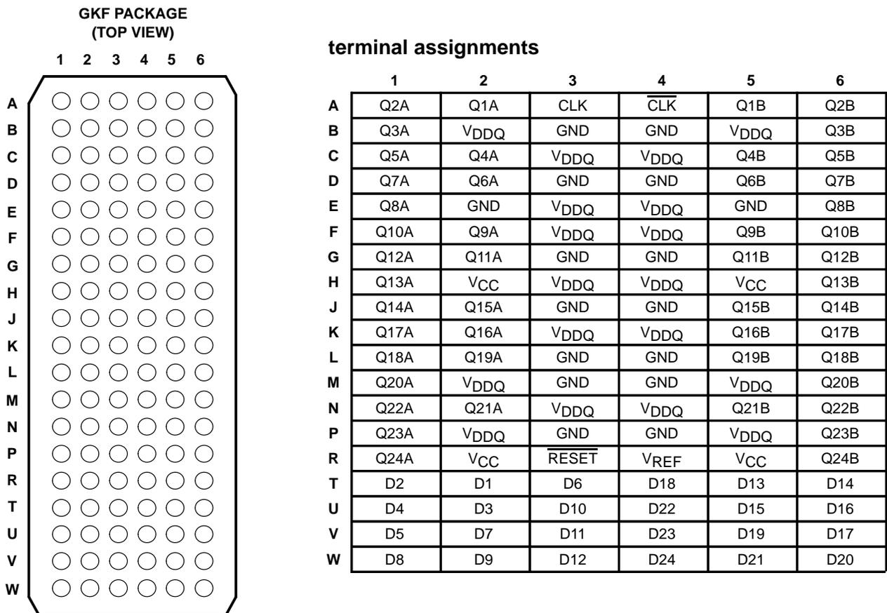
Figure 3. SN74SSTV32852 GKF Package Pinout and Terminal Assignments
