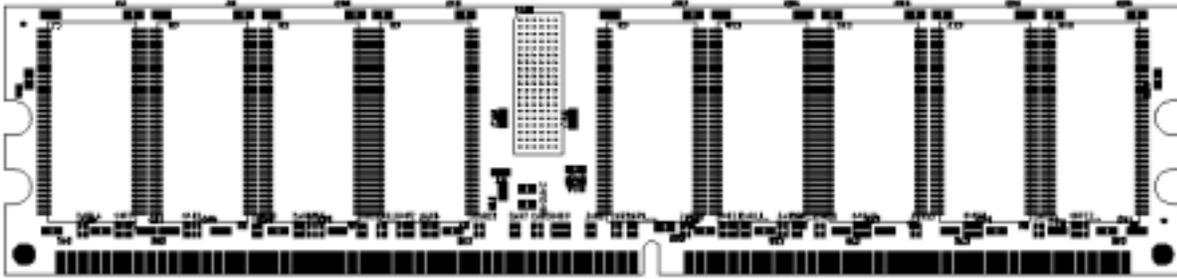
**Figure 7. Other Side of DIMM With SN74SSTV32852 Mounted**
