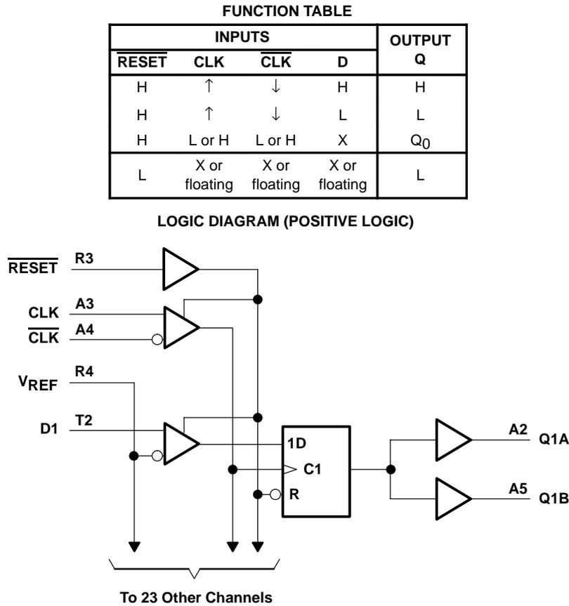
**Figure 4. Function Table and Logic Diagram of SN74SSTV32852**
