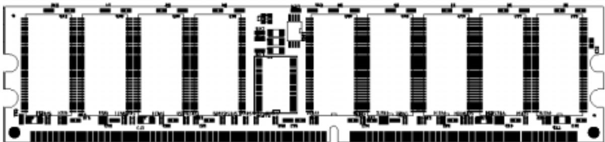
**Figure 6. One Side of DIMM With SDRAMs, PLL, and SPD Mounted**
