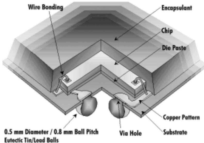
**Figure 11. LFBGA Cross Section**
