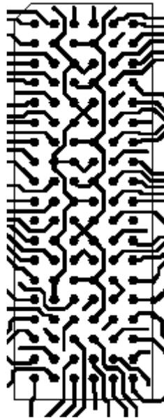
**Figure 8. Example Routing of SN74SSTV32852 Register**
