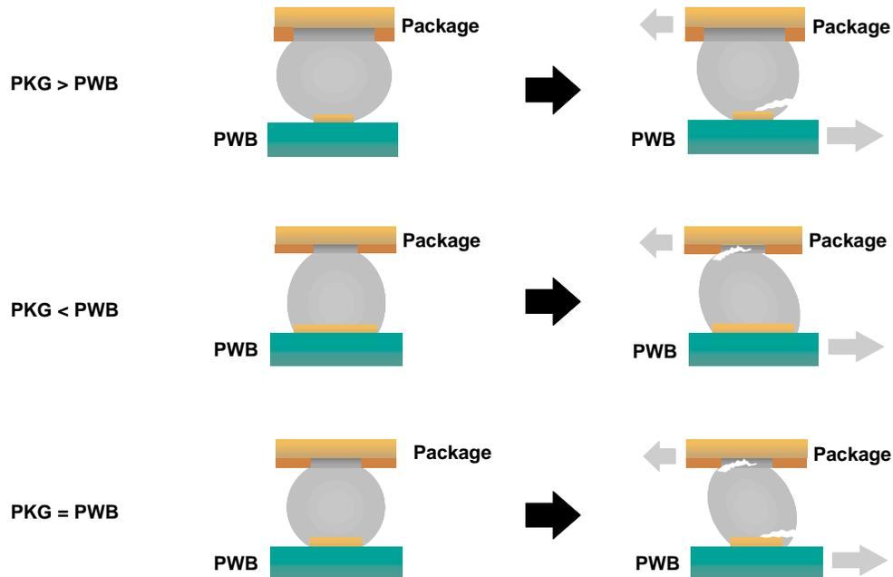
**Figure 13. Solder-Ball Behavior During Thermal Cycling**
