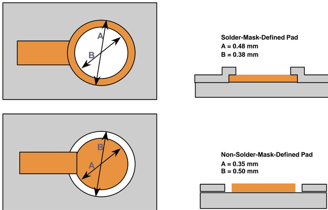
**Figure 14. Land-Pad Dimensions for 114-Ball BGA Package**
