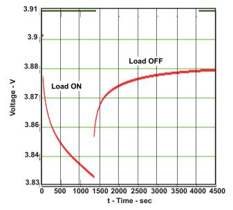
Figure 4. Battery Cell Voltage Waveform During Discharge and Relaxation Mode
