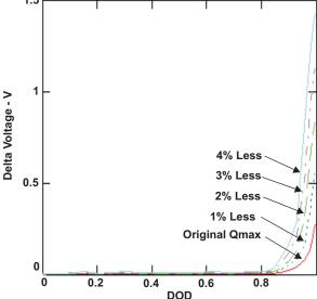
(b) Resulting voltage differences between the cells
