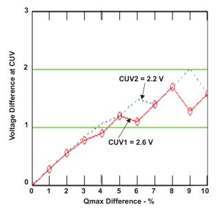
Figure 3. The Relationship Between the Cell Voltage Difference at Cell Under Voltage and Q<sub>max</sub> Difference
